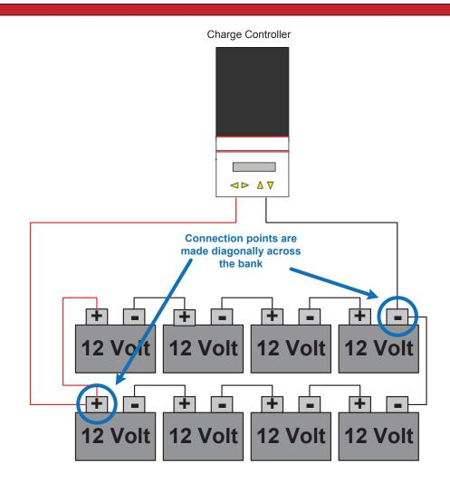
**IMPORTANT:** This is not intended to be a complete system diagram; fusing, disconnects, and grounding should comply with local electric codes.
