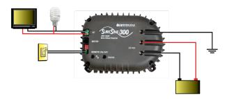
high temperature and low voltage disconnect. Recovery from most faults is automatic
