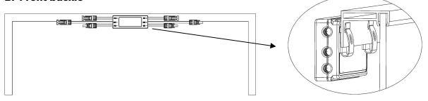
NOTE: Do not place the RSD-D (including DC connectors) where exposed to the sun, rain or snow, even gap between modules. Allow a minimum of 3/4"(1.5cm.) between the roof and the bottom of the RSD-D to allow proper air flow.
