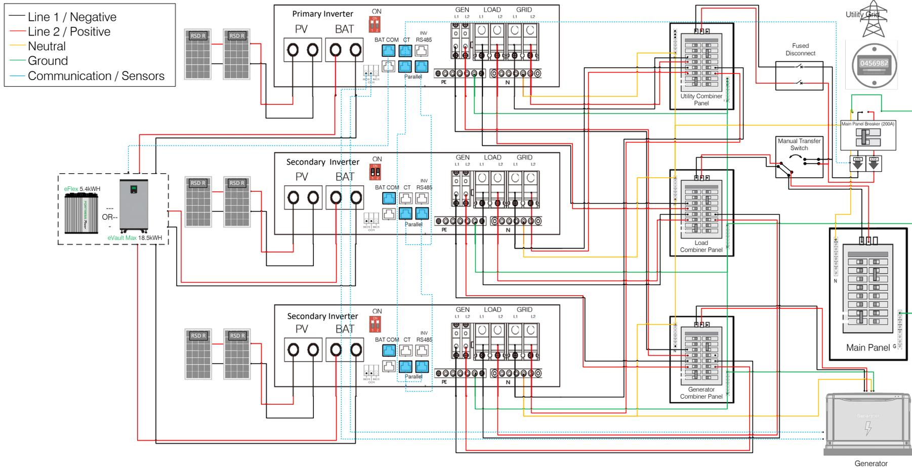
**There should be only one Neutral to Ground Bond established on the supply side of the electrical system.**
