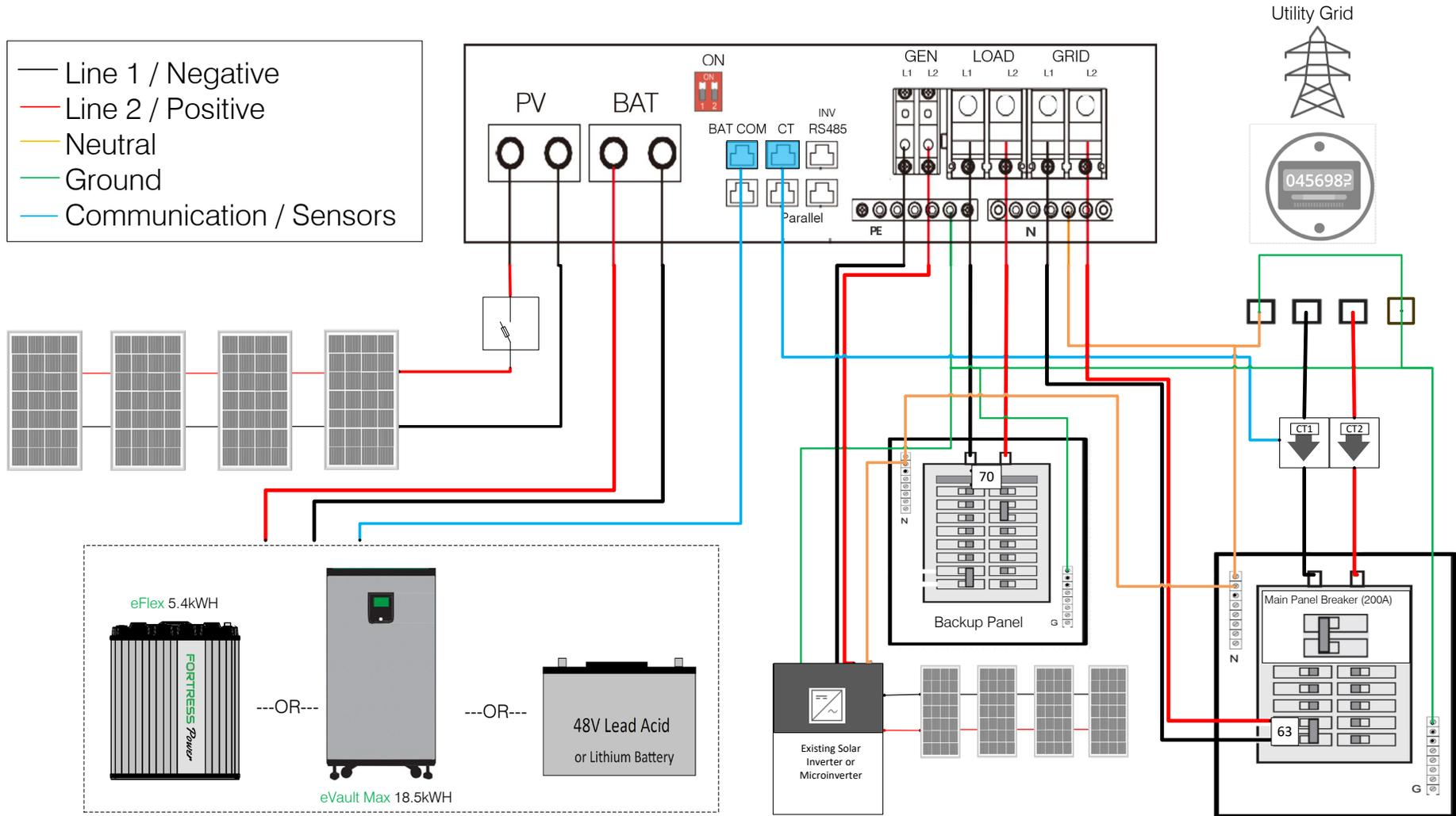
**There should be only one Neutral to Ground Bond established on the supply side of the electrical system.**
