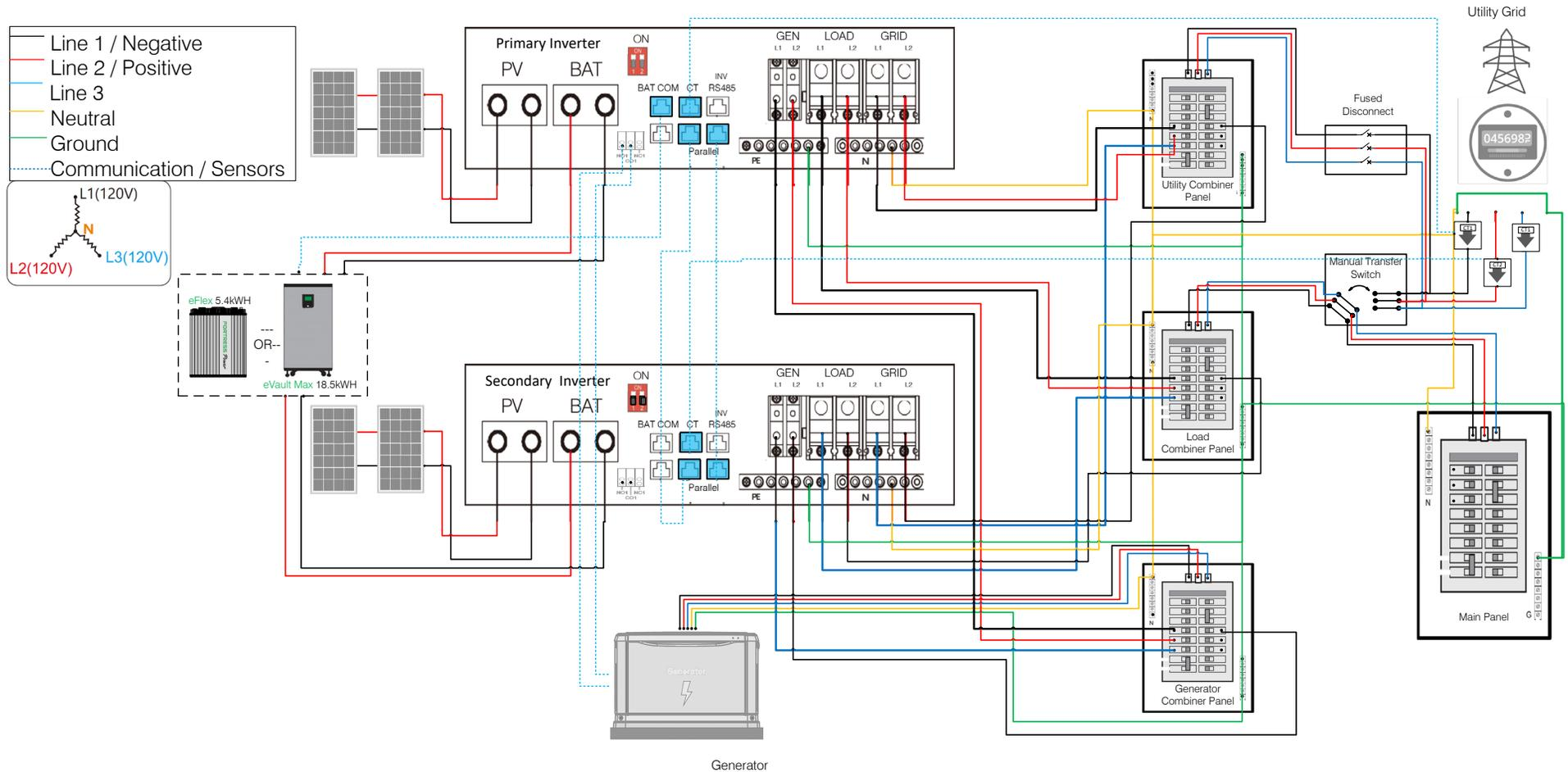
**There should be only one Neutral to Ground Bond established on the supply side of the electrical system.**
