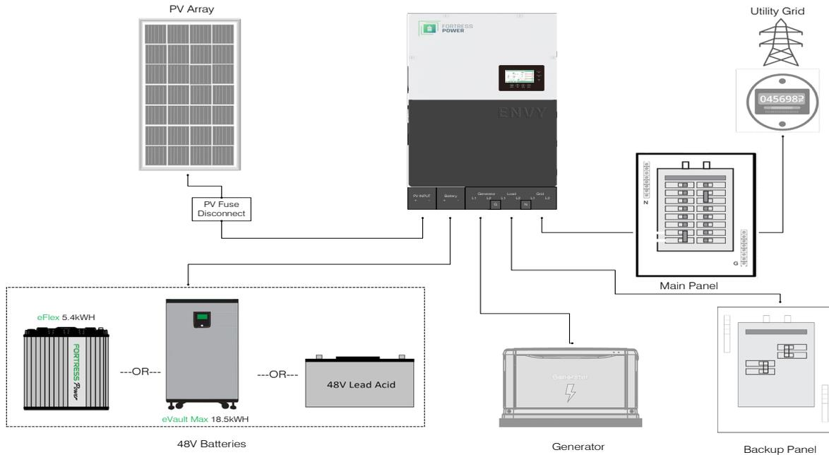
The Envoy 8k has already built in breakers for all AC connections as well as the Battery connection. Please include the following PV Fuse breakers in accordance with the local jurisdiction.
