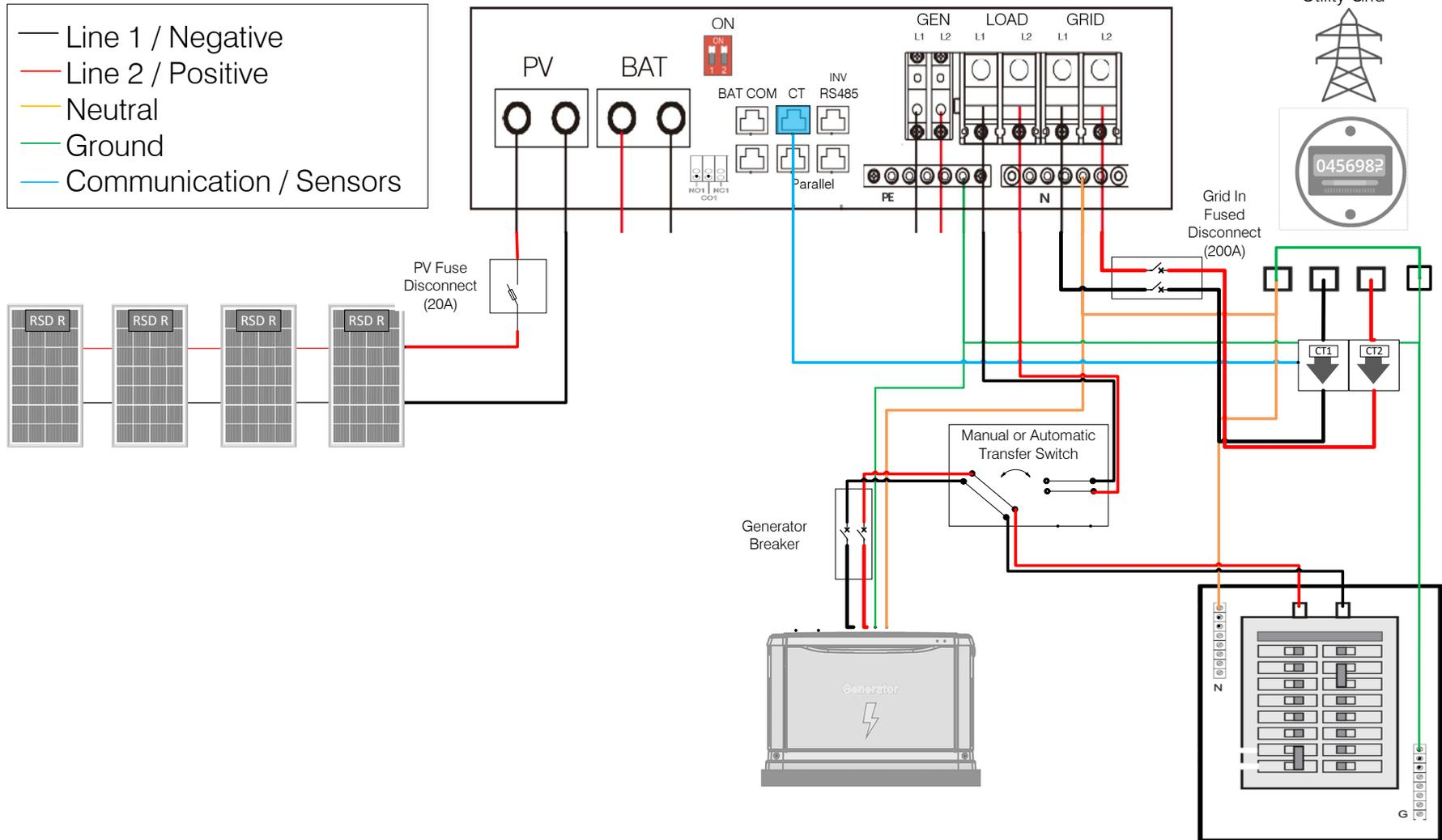
**This schematic includes an optional generator addition in the case of grid outage. Note: the internal RSD transmitter is powered by a 12V source that is converted and supplied by grid connection or battery connection. Grid outage will deactivate the RSD transmitter.**
