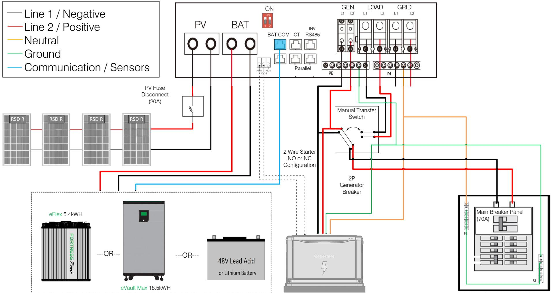
**There should be only one Neutral to Ground Bond established at the Load Panel of the electrical system.**
