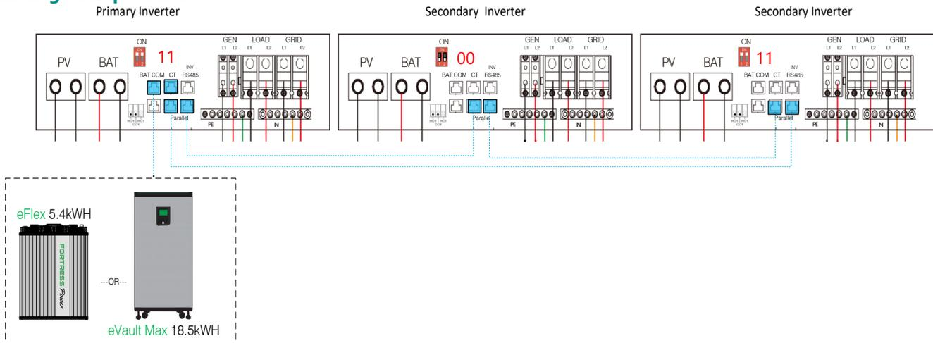
Use the Communication Cables included in the in the Envy Inverter along with those of the **eFlex5.4kWh** and **eVault Max 18.5kWh**. The Envy paralleling communication cables measures 6.5ft. Therefore, installers might need to provide an extra longer communication cable to be able to make parallel connections if installed further apart. The battery communicates only with the Master Inverter through Modbus RS485.
