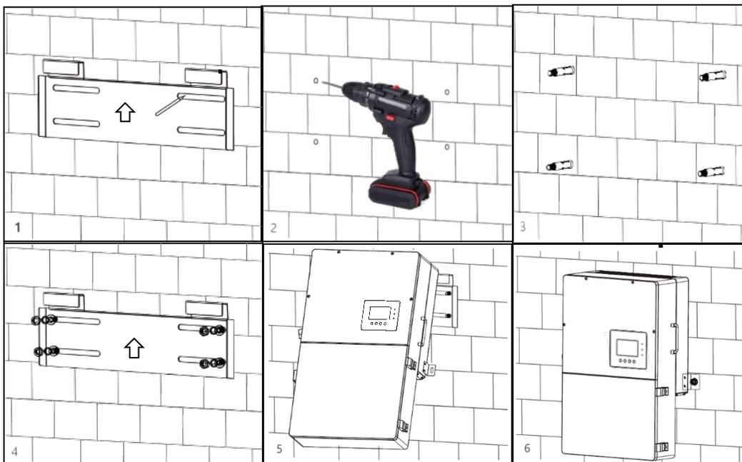
1. Mark the drill holes positions with the mounting bracket,
