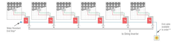
\* Water resistant end stop - Insert the two red sealing plugs in to the Tyco Superseal plug (supplied) and connect to the DC output connector of the last FireRaptor (FRS-01/FRS-02) in the series installation. If only a single FireRaptor (FRS-01/FRS-02) is used then this part is still used to seal the DC output connector.
