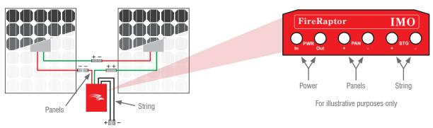
Connect the FireRaptor's two output cables to the DC isolator/Solar Inverter ensuring that the correct polarity is maintained throughout the electrical wiring.
