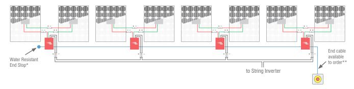
If the array has an odd number of panels, a single panel can be connected directly to the positive (+) and negative (-) panel cables of the FireRaptor.
