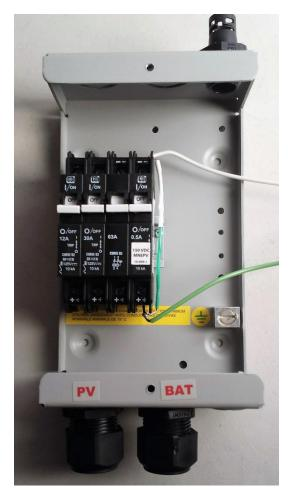
**(HINT)** When stripping wire, it is recommended to only strip enough insulation off the wire to fit into your connecter, approximately 3/8" for this breaker and for the negative busbar.
