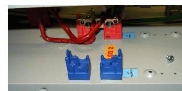
Position new mounting blocks as shown. Secure them with screws removed earlier*
