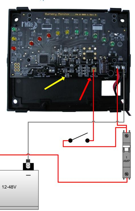
To modify an MNBCM for Key Switch operation, simply remove the "zero ohm" resistor #28 as indicated by the yellow arrow and solder a small gauge wire (#16-22) to the pad indicated by the Red Arrow and labeled "KEY SWITCH".
