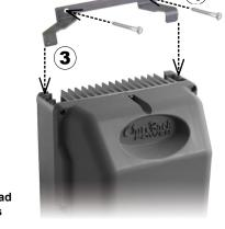
Bracket hole spacing: 5.13" (13.0 mm) Vertical space between upper and lower bracket holes: Approximately 20" when mounted
