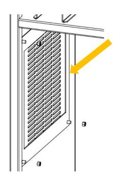
Screw the nuts and insert the filter from the gap between the mounting plate and the main body. 3 Tighten the nuts.
