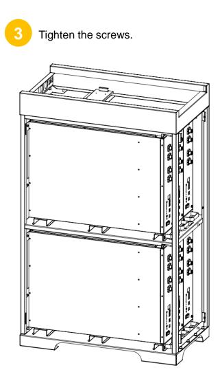
Fix the batteries to the main body with screws.
