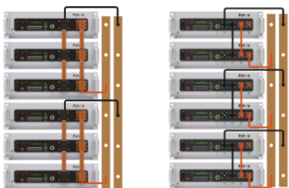
Figure 5-1 Schematic diagram of power cable connection
