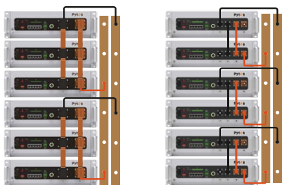
Figure 5-1 Schematic diagram of power cable connection
