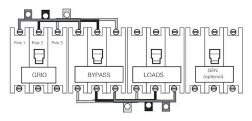
4. Connect the AC wiring as shown in Figure 57.
