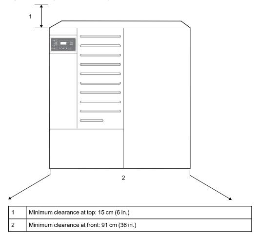
Figure 13 Example of clearance requirements for a Conext XW Pro with PDP
