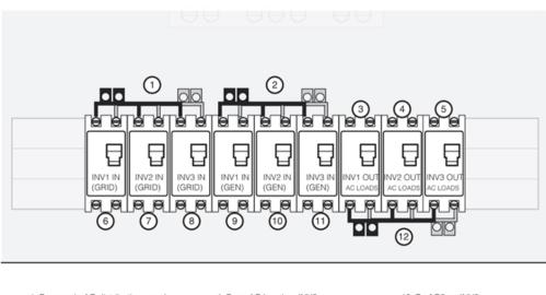
1. From main AC distribution panel or transfer switch NOTE: Install L1 power distribution bar (jumper) in first GRID/GEN
