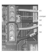
Secondary transformer wire X1, X2, X3, and X4 locations AFTER reconfiguration
