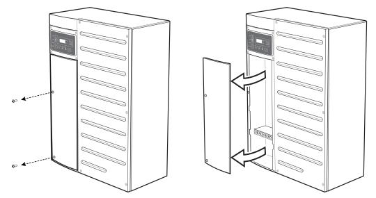
Figure 24 AC access panel removal (internal components hidden for clarity)
