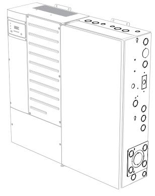
Figure 14 Example of available knockouts on the PDP
