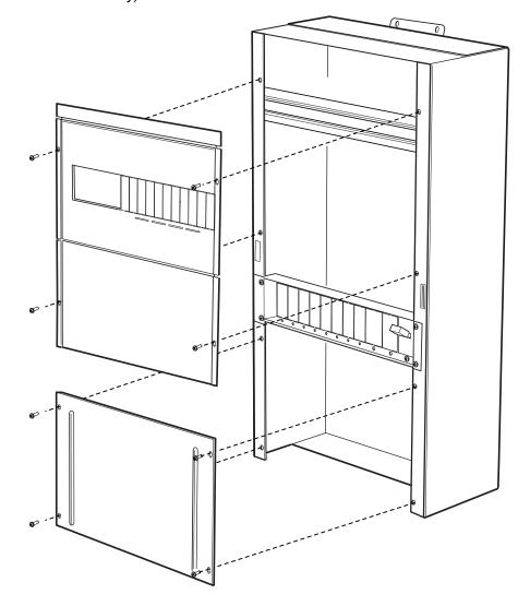
Figure 25 Power Distribution Panel (PDP) faceplate removal (internal components hidden for clarity)
