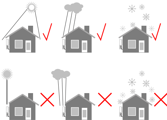
Figure 14 Inverter exposure requirements
