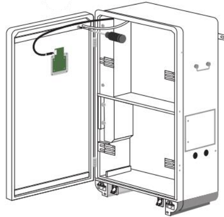
Figure 15 Display cable and ground connection
